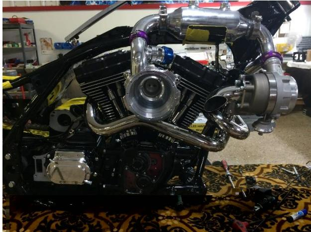
Liquid/Air intercooler making this one of a kind system truly unique. Our "heat-sink style" plenum intercooler works great for all your typical riding conditions, while our liquid cooled option is more for the speed freak really looking to run the motor hard and aggressive, i.e. "Under high boost for extended periods of time".
